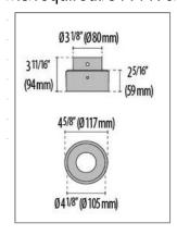
Base cover shape and bolt circle diameter (BCD) will vary based on pole size and vendor. Contact factory for details related to your project.
